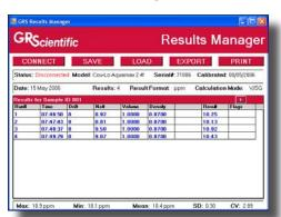
This is a windows application that allows you to view and print sets of results created by the Cou-Lo Aquamax KF Moisture Meter. It can download results directly from the titrator through a serial
